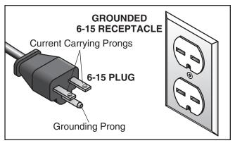
Figure 1. Typical 6-15 plug and receptacle.
